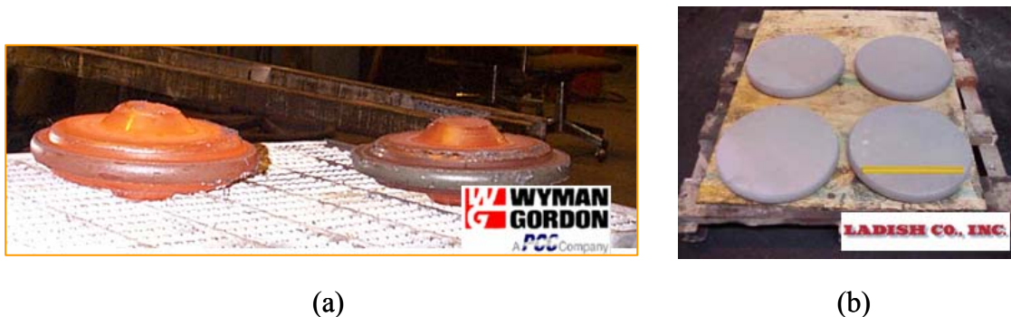
Figure 9. (a) Sub-scale disc forgings produced by Wyman Gordon Houston. (b) Pancake forgings produced by the Ladish Company.
