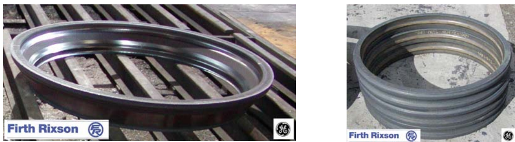
Figure 8. Full-size component ring-rolled forgings of Allvac ® 718Plus ® Alloy produced in the MAI Low Cost High Temperature Structural Material program [12].
